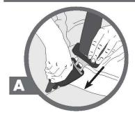
BUCKLE the latch plate into the matching buckle after pulling out the shoulder belt webbing from the seatback. LISTEN for the CLICK sound when the latch plate is fastened!
