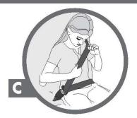
TIGHTEN the lap portion by pulling upward on the shoulder belt. Be sure that the shoulder belt is snug across the chest and crosses the center of the shoulder.
