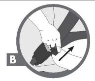
CHECK that the buckle connection is secure by tugging firmly on the seat belt latch plate.
